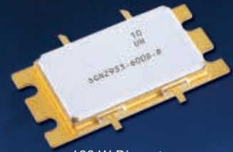
600 W Discrete 2.9 - 3.3 GHz G_p = 13 dB 50 \Omega Matched Pair
